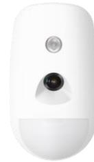
PIRCAM is a high speed bus detector with built-in high quality camera which can provide an ideal solution for video verification via motion pictures transmitted to an ARC or to personal phones via APPs.
